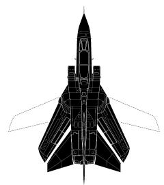
The Tornado stands as a top all-weather, day-night, supersonic fighter-attack aircraft. It was developed and built by the tri-nation Panavia consortium created by Britain, Germany, and Italy. It was, at its outset, one of the few tactical aircraft able to attack at very low level, at any time, in any kind of weather. However, this fighter has done more than strike alone. Tornado variants also have been optimized for electronic combat and air interception, plus maritime missions.
